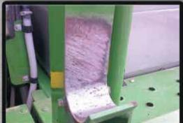
Boom Nest Guards protects the boom and cradle from excessive wear.
