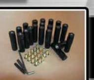
Durable powder coated spacers fasten to the remaining wheel studs that protrude beyond the wheel nuts and are machined to extend beyond the end of the hub providing a sturdy mounting surface utilizing our custom zinc coated mounting hardware.
